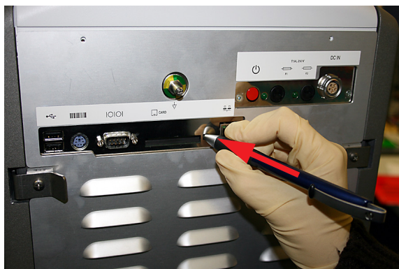
A Press the ejecting device using a pen.
