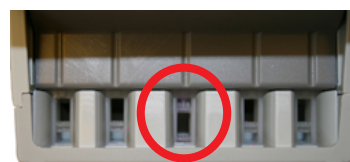
B Incorrect valve position (3rd valve center)
