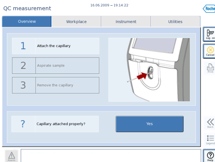
Figure D-55 Attach the capillary
