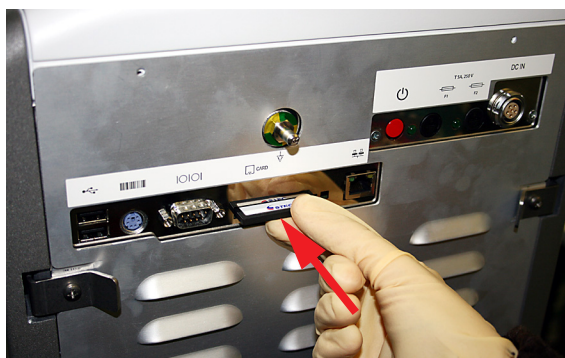
Figure F-12 Inserting the CompactFlash memory card
