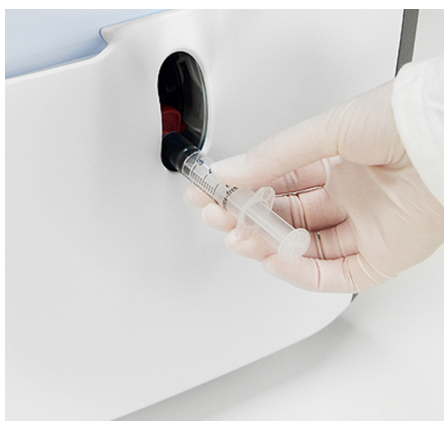
Figure D-17 The syringe is plugged in at the fill port.
