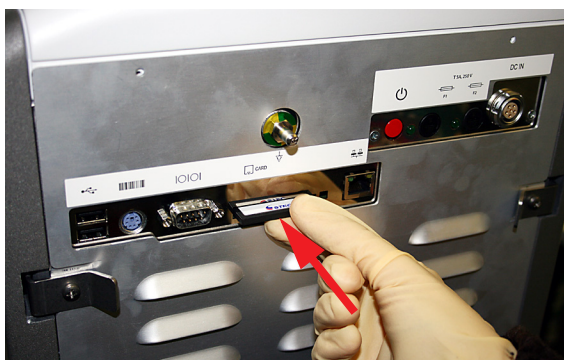
Figure F-21 Inserting the CompactFlash memory card
