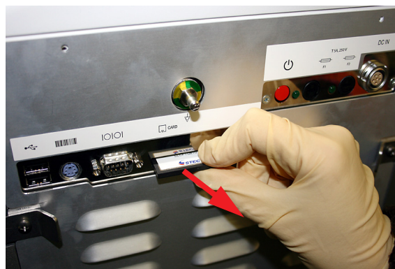
B Remove the CompactFlash memory card
