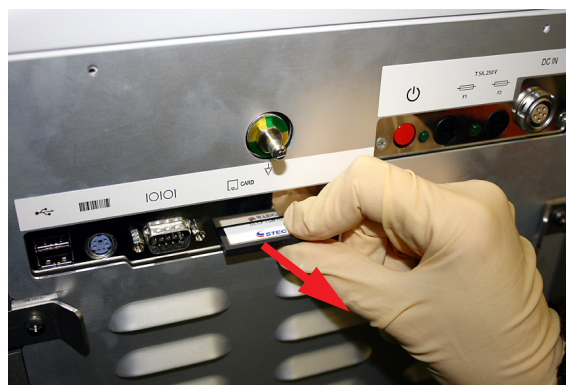
B Remove the CompactFlash memory card
